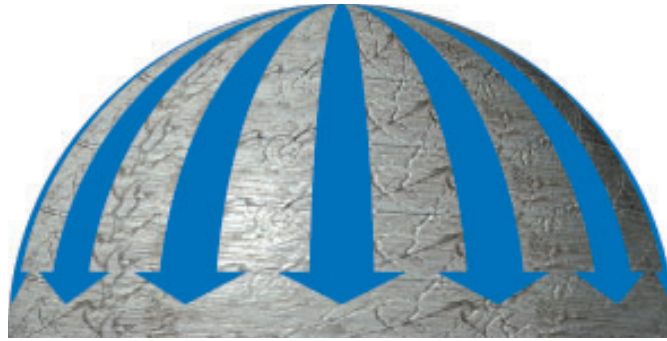
Figure 9 The compression force on this dome is directed downward in many planes at once.
