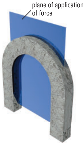
Figure 8 The compression force on this arch is directed downward in a single plane.
